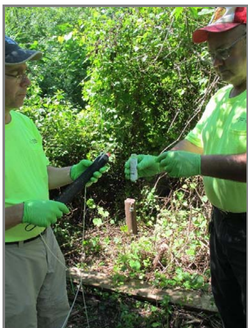
Charlie pours and Carl fills and tops off the meniscus. It's a requirement for VOAs that there be no bubbles.
