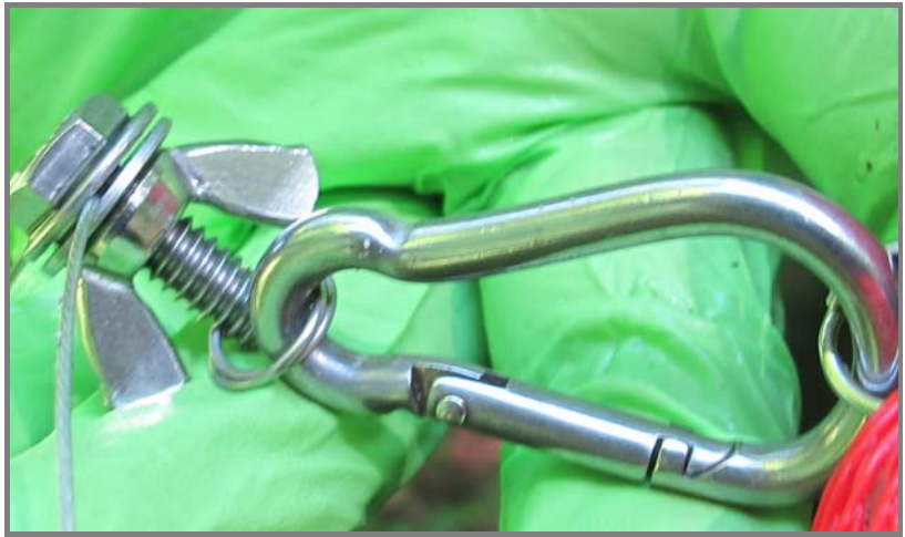
Wire-hung permeable bag. The remedial callout contractor AZTECH made the hanging attachment. The short bolt is drilled at the top and bottom.
