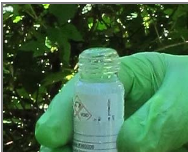
Charlie pours and Carl fills and tops off the meniscus. It's a requirement for VOAs that there be no bubbles.
