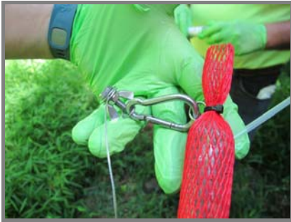
Wire-hung permeable bag. The remedial callout contractor AZTECH made the hanging attachment. The short bolt is drilled at the top and bottom.
