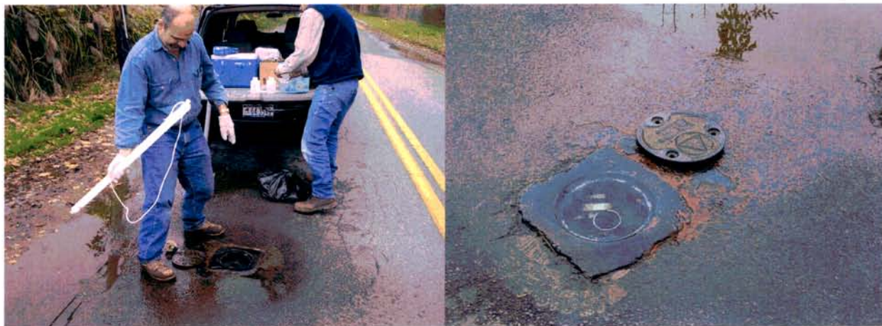
Figures 8a and 8b. Sample 9 was collected from monitoring well 2S, a flush-mounted well installed in the road surface of Taylor Lane just west of the landfill. This well, and three other nearby monitoring wells were observed to be in a continuously flowing (artesian) state. Sample 10 was a solid sample of iron-stained (gray) soil collected from a leachate seep zone in the road shoulder (east side) of Taylor Lane.
