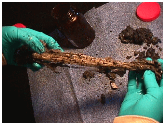
Elastic Material of Highly Concentrated PCBs (sample collected from Operable Unit #1)
