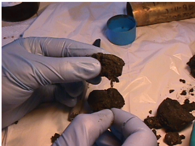
Hair-like Filament of Elastic Material (sample collected from Operable Unit #1)
