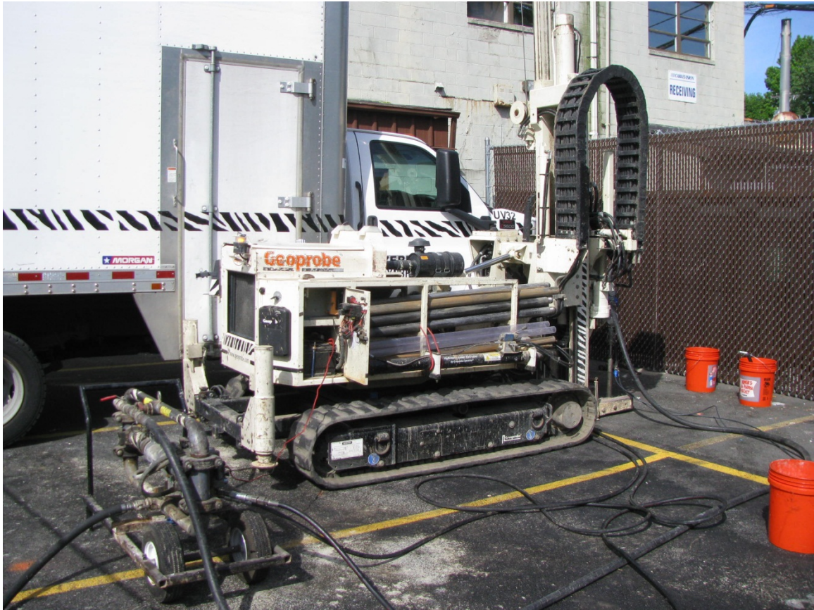
PHOTOGRAPH OF GEOPROBE DRILL RIG USED FOR 2014 REMEDIAL INJECTIONS.
