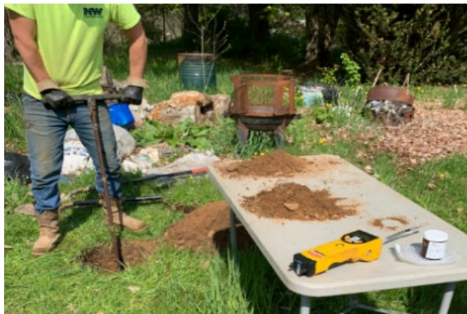
Example of hand auguring equipment
