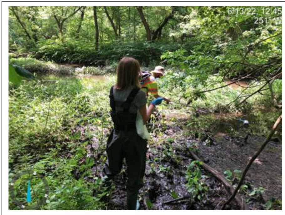
Photograph 3: View of START V collecting a surface water sample, utilizing a dedicated dip sampler lined with a poly bag, from Property RMP. Sample was transferred to two 250 mL poly bottles for total and dissolved mercury analysis.
