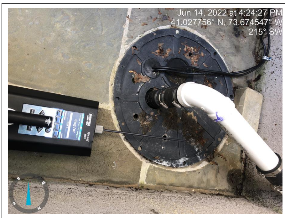
Photograph 34: View of air monitoring conducted with a Jerome 505. A reading of 0 ng/m 3 was detected at Property P047 near the rear entry to the basement. No sampling was conducted at this location, due to lid being fastened to top of sump pump.
