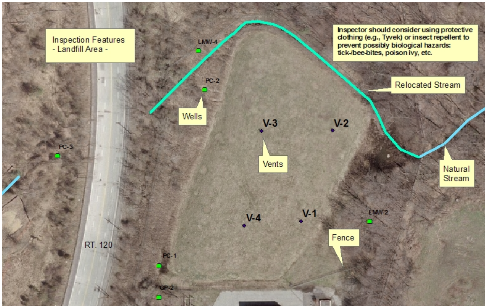
Landfill Inspection Features
