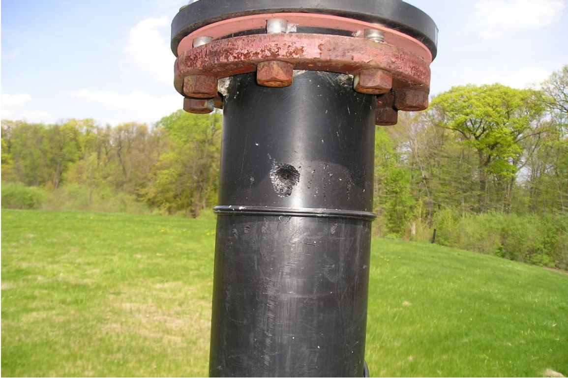
Photo 21: Pinhole in V-1 from suspected insect boring
