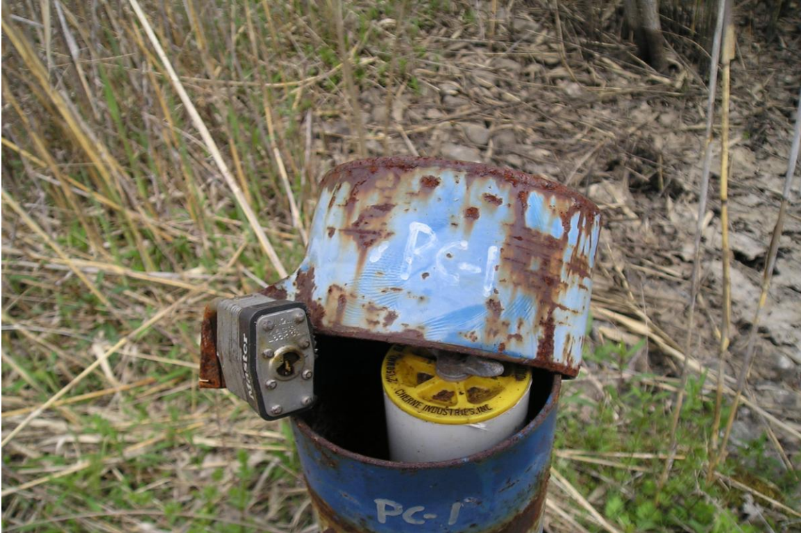
Photo 7: Well PC-1 with broken key in lock)
