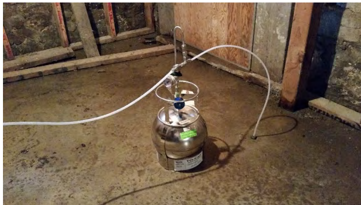
Photograph 6 – Sample collection at temporary sub-slab vapor point
