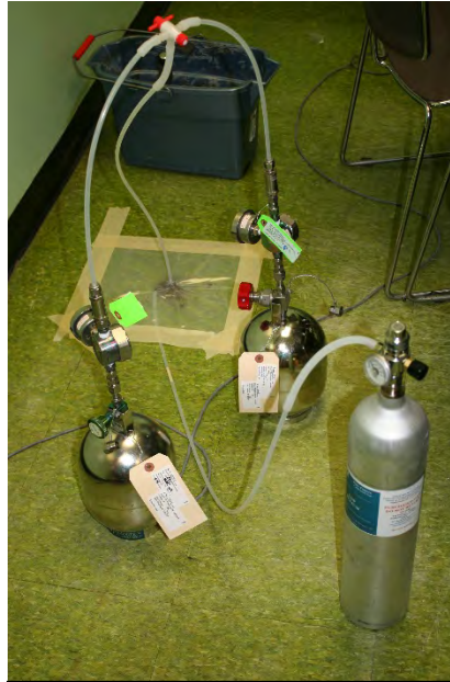
Photograph 15 - Field duplicate sample collection setup
