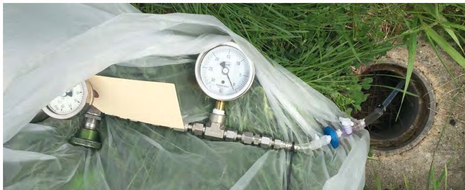
Photograph 18 – Exterior soil gas sampling point with moisture filter setup to begin shut-in leak test
