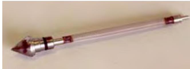
Photograph 7 – Stainless-steel mesh soil vapor point
