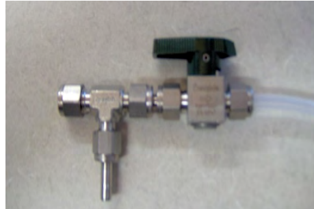
Photograph 17 - T-connection for quantitative tracer gas testing
