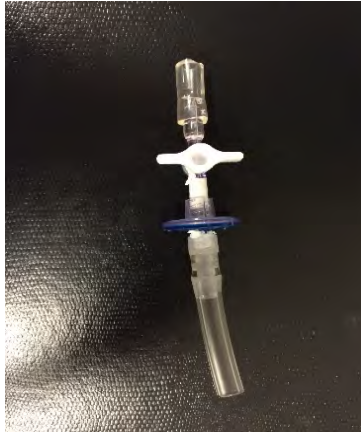
Photograph 9 – In-line moisture filter and stopcock assembly (See Photograph 13, Item [C])
