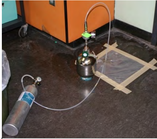
Photograph 21 - Plastic wrap leak detection method during sampling
