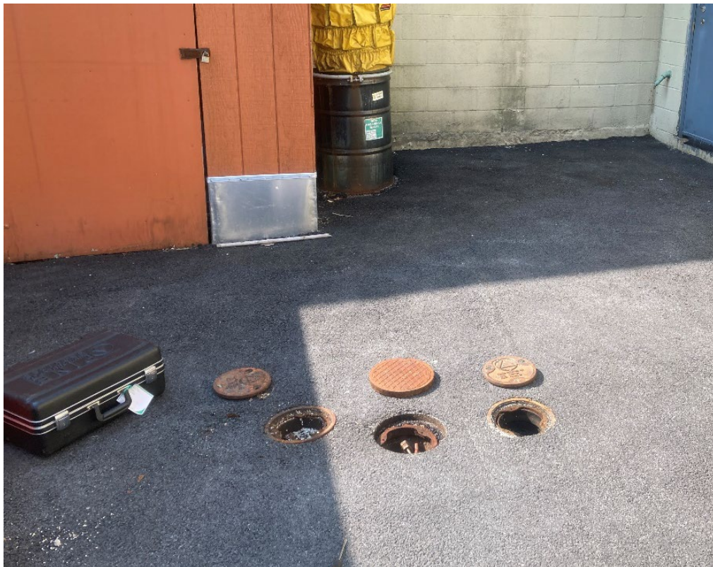
Photograph 2: View of monitoring wells behind Singas Pizza.
