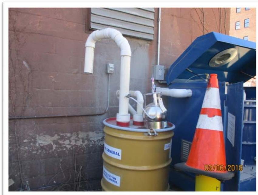
**2. Air Sampling at the Discharge of the Carbon Vessel
