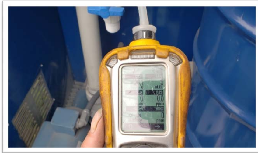
3. A Typical PID Reading by Using MultiRAE
