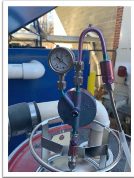
1. Air Sampling at the Discharge of the Blower by Using Suma-Canister
