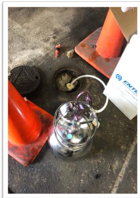
2. Air Sampling at the SVE Points by Using Suma-Canister
