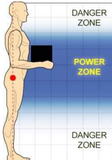
Figure 1: Lifting Power Zone
