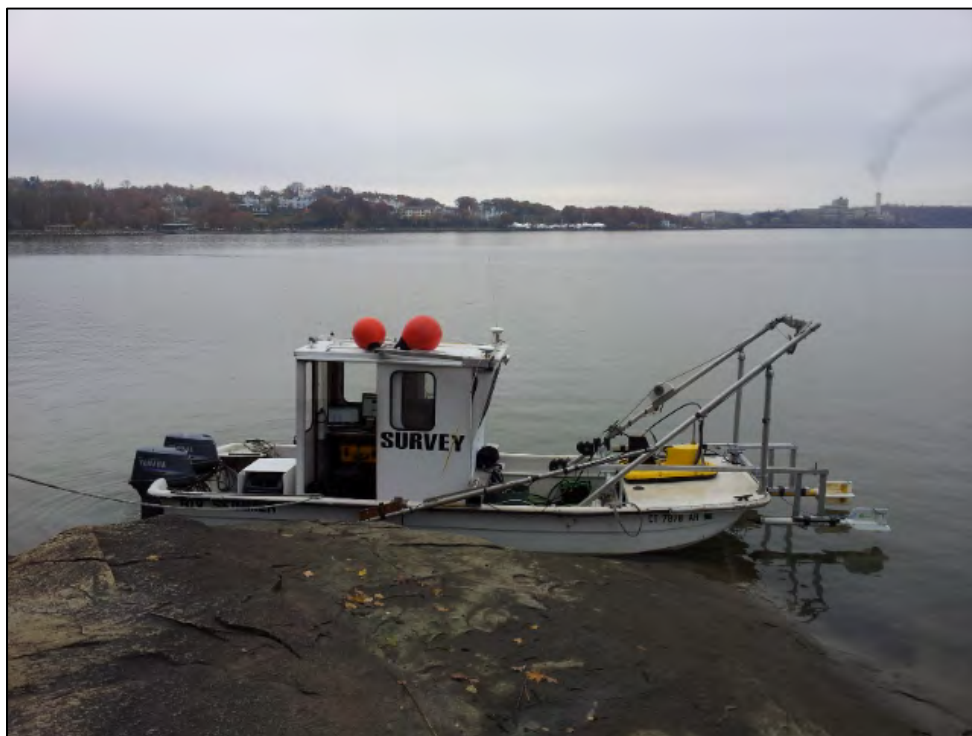
Figure 2. Shallow draft vessel R/V Skimmer used for survey operations.
