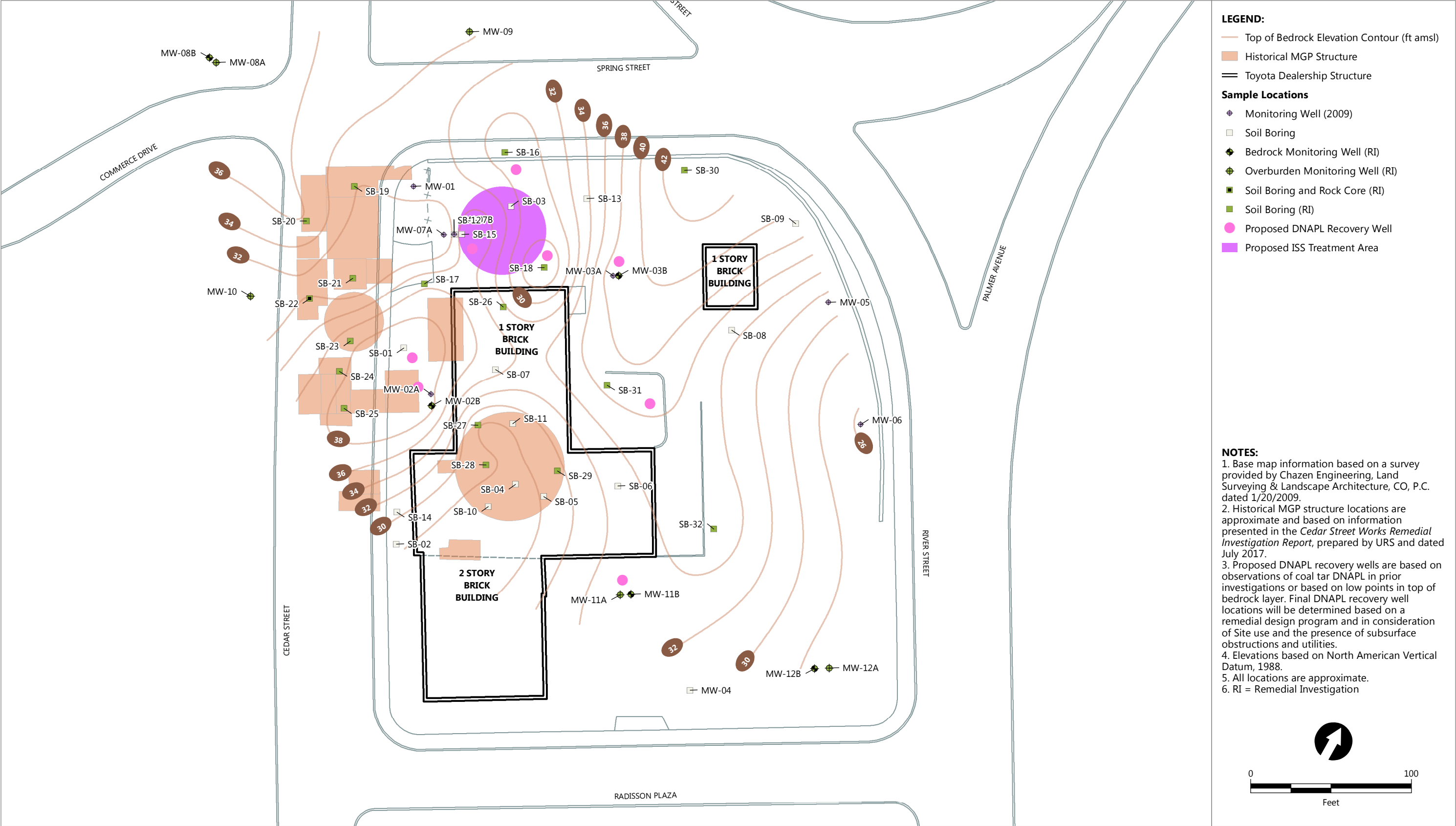
Figure 5-2 Proposed Remedial Alternative 3: ISS of North Gas Holder, DNAPL Recovery, Maintain Existing Surface Covers, Groundwater Monitoring, and Institutional Controls Cedar Street Works Former Manufactured Gas Plant Site - Alternatives Analysis Report Consolidated Edison Company of New York, Inc.
