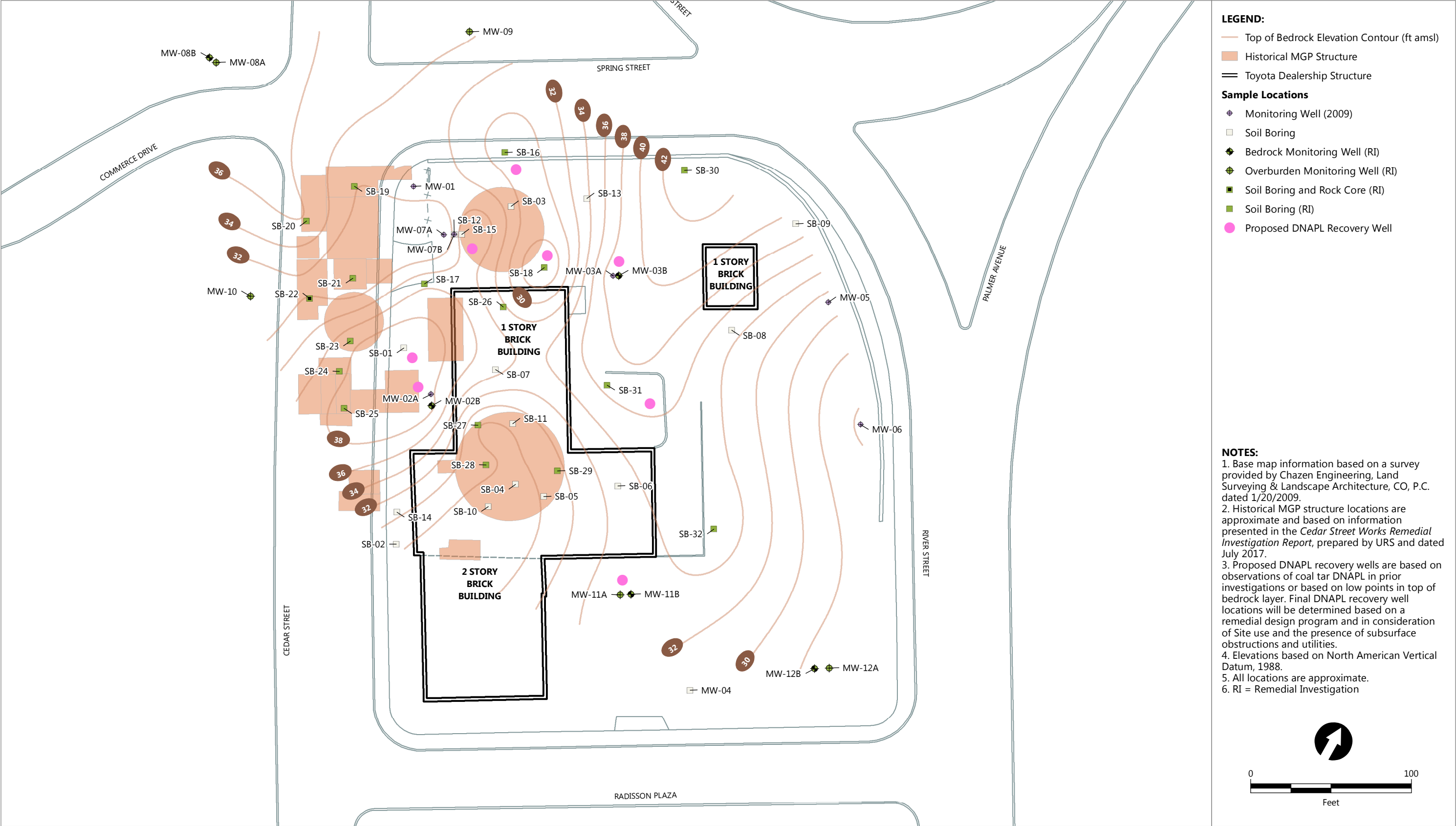
Figure 5-1 Proposed Remedial Alternative 2: DNAPL Recovery, Maintain Existing Surface Covers, Groundwater Monitoring, and Institutional Controls Cedar Street Works Former Manufactured Gas Plant Site - Alternatives Analysis Report Consolidated Edison Company of New York, Inc.
