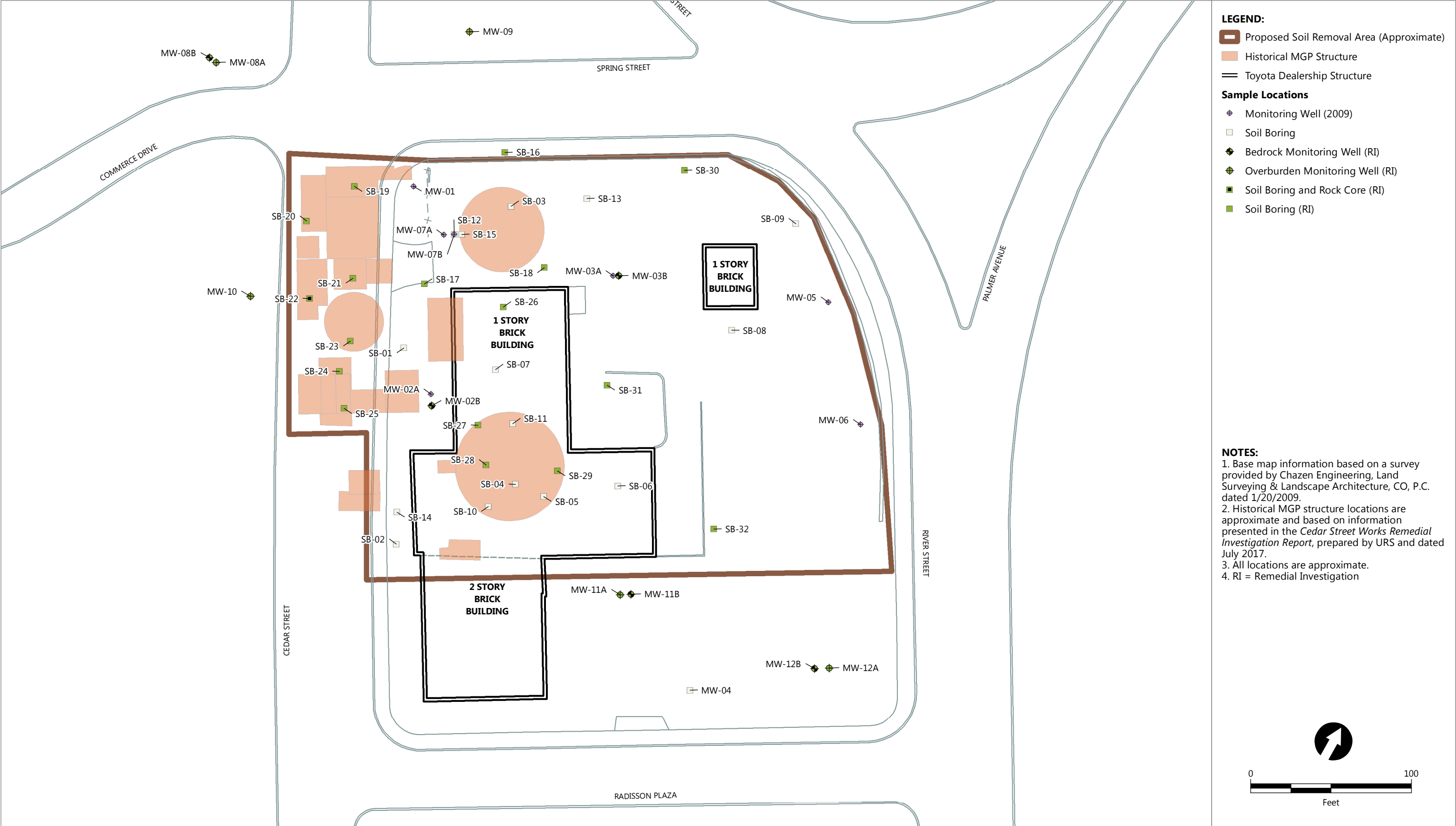
Figure 5-3 Proposed Remedial Alternative 4: Soil Removal, Groundwater Monitoring, and Institutional Controls Cedar Street Works Former Manufactured Gas Plant Site - Alternatives Analysis Report Consolidated Edison Company of New York, Inc.
