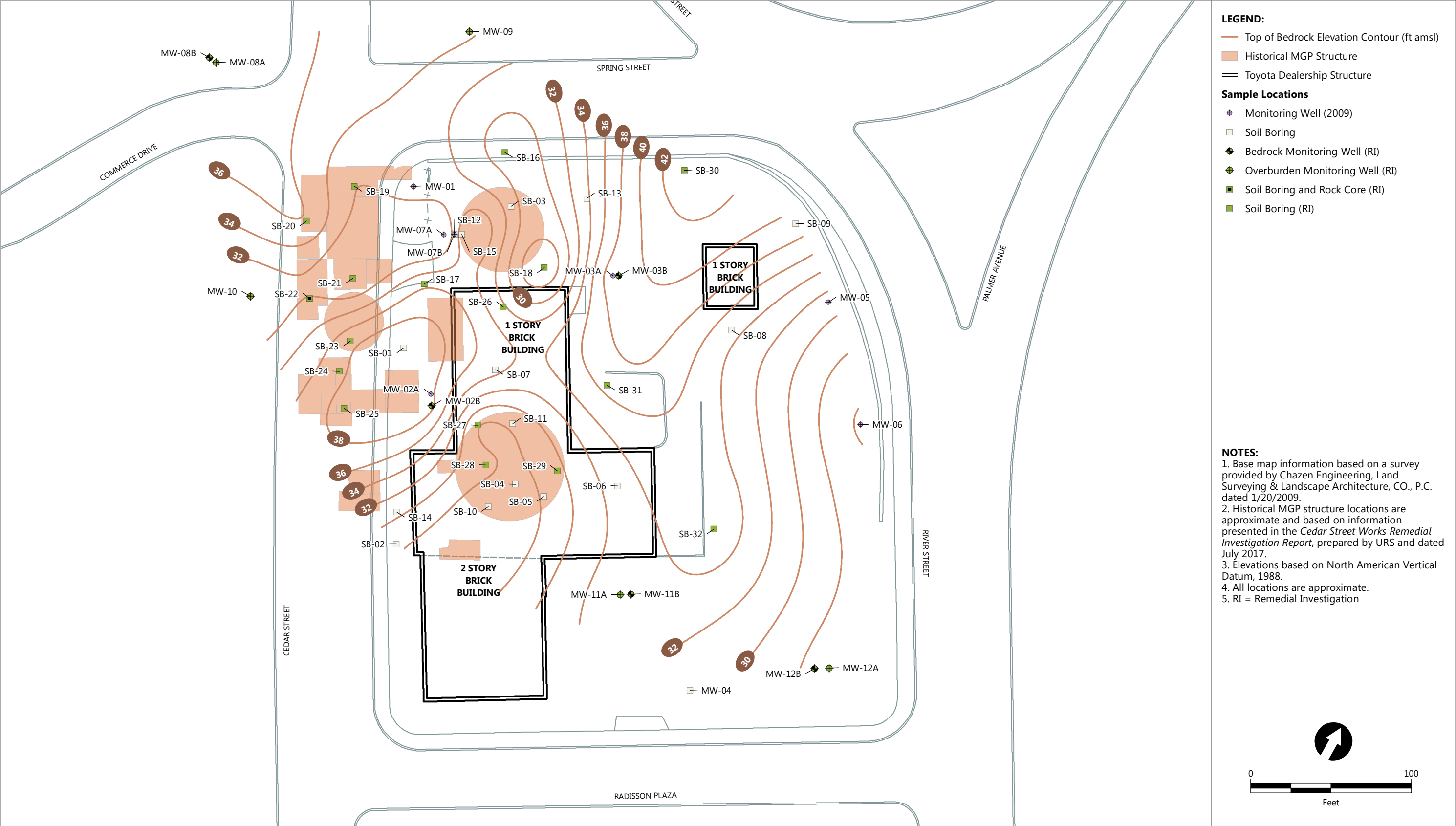
Figure 1-5 Estimated Top of Bedrock Surface Cedar Street Works Former Manufactured Gas Plant Site - Alternatives Analysis Report Consolidated Edison Company of New York, Inc.
