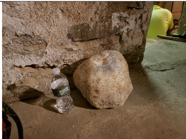
Boulder removed from approximately 1 foot below the slab after concrete coring at DP-18.
