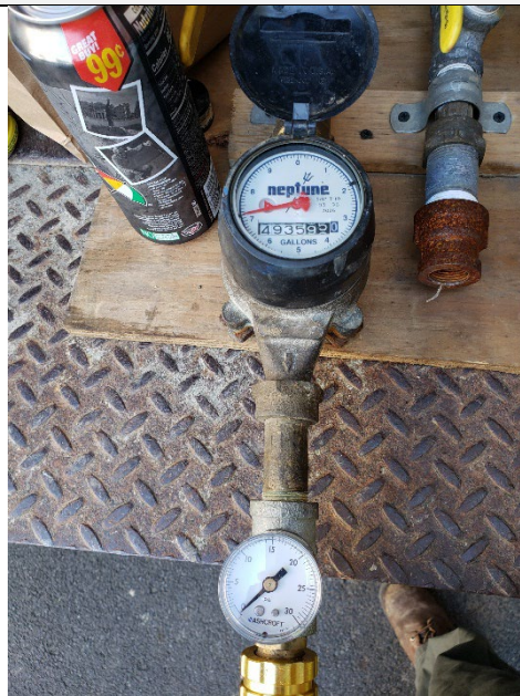
Flow meter and pressure gauge installed downstream of water tank for injection testing.
