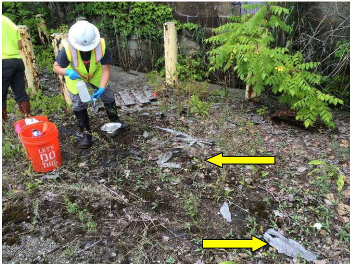
Photo 2. Bulk Galbestos on the ground surface
