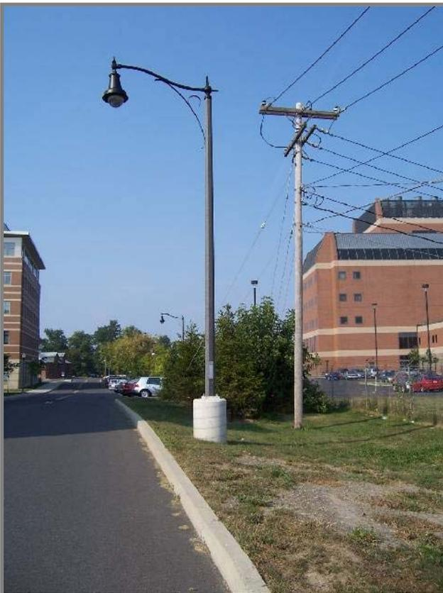
Photo left. We'd like to locate a well in the green shrubs, center of the picture. The location is to be between the curb and the fence, not too deep into the shrubs, closer to the curb than the fence. The shot shows that there are overhead wires to keep clear of and there likely is a buried electric line to the light pole.
