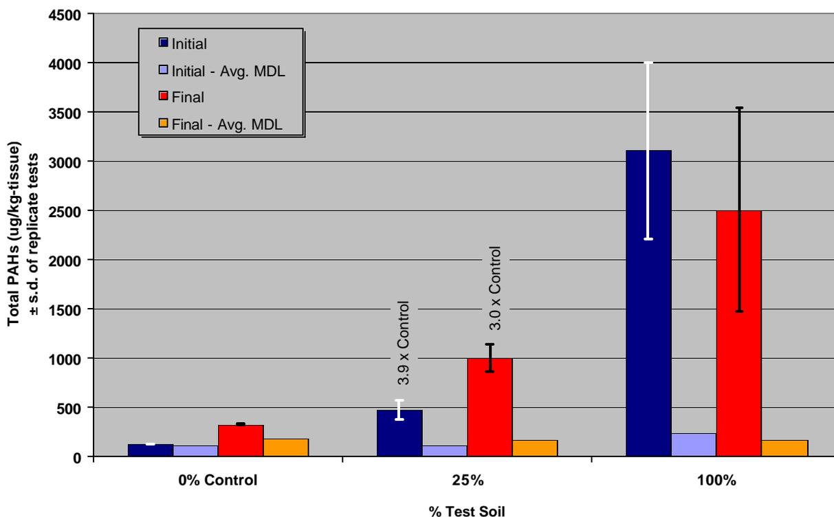
**Figure 18: 28-Day Earthworm Bioaccumulation Test Analytical Results**
