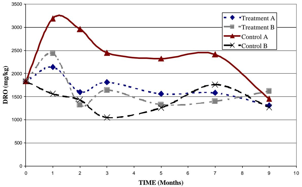
**Figure 8: DRO Results from Soil-column Evaluation**
