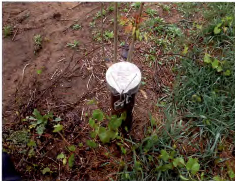
Photograph 3. Monitoring Well MW-9 located at the west end of the site, north of the rail road tracks.
