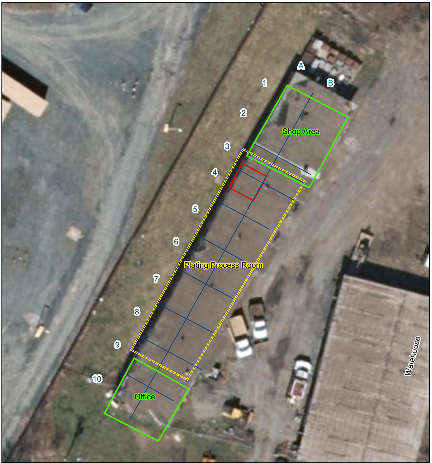
Figure 9 Approximate Extent of Hexavalent Chromium Impacted Building Material Basis of Design Report Perfection Plating Site (4-01-037) Watervliet, New York
