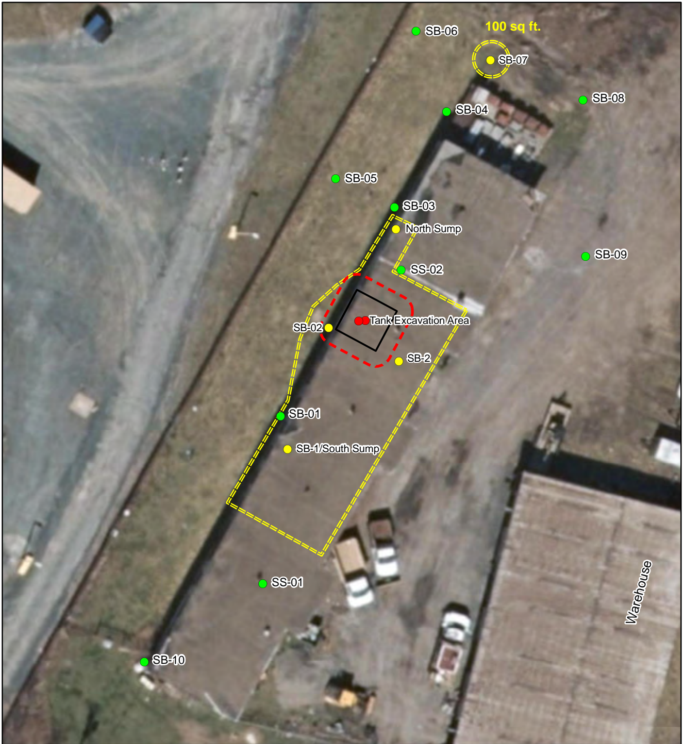
Figure 10 Approximate Extent of Hexavalent Chromium Impacted Soil Basis of Design Report Perfection Plating Site (4-01-037) Watervliet, New York
