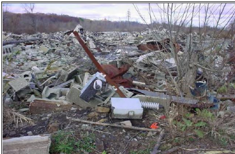
Photograph 2: Abandoned capacitors. Underlying soil PCB concentrations exceeded hazardous waste thresholds (2007).
