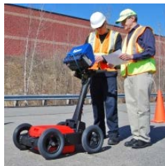
Figure 1: Ground Penetrating Radar equipment.
