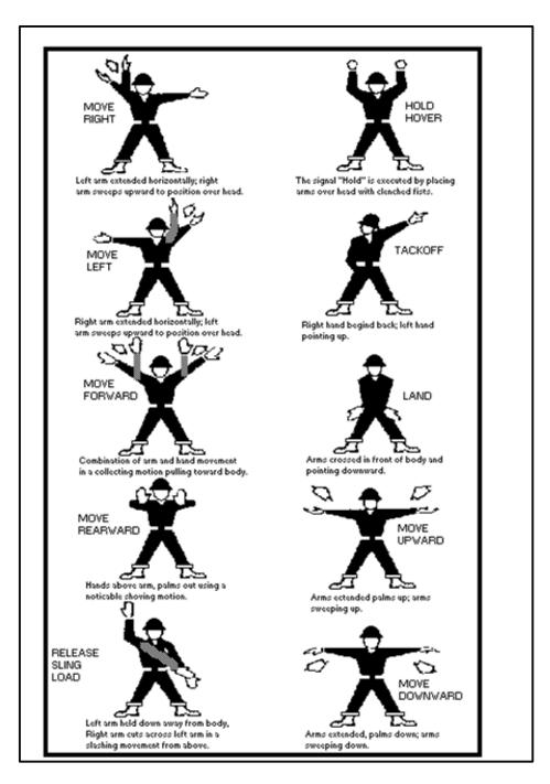
Figure 5-2 Helicopter Landing Hand Signals
