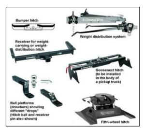
Figure 3-2 Types of Trailer Hitches
