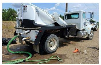
Vacuum trucks that do not have automatic vacuum relief may implode if the vacuum is exceeds the operating limits of the vessel.
