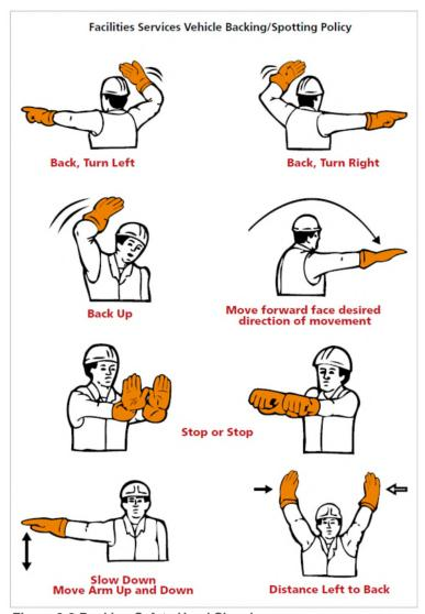
Figure 3-3 Backing Safety Hand Signals
