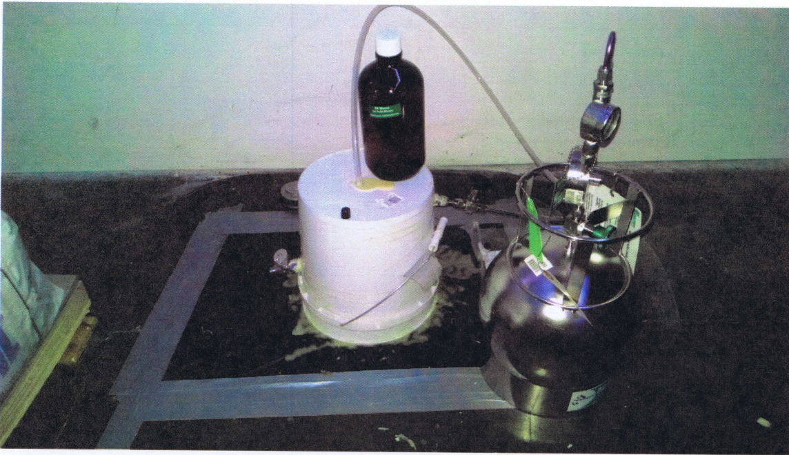
Figure 1: Sub-Slab sampling point (DB-VMP-2).
