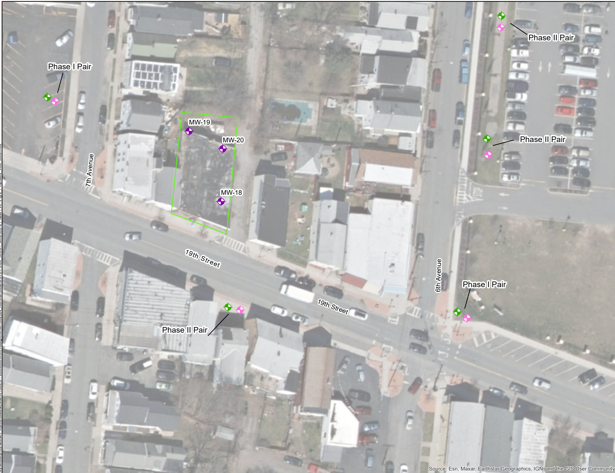
Figure 5 Proposed Bedrock Well Locations OU-2 Phase I Work Plan Admiral Cleaners Watervliet, Albany County, New York
