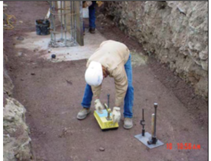
Picture No.: 044 Date Taken: October 10, 2002 Description: Compaction testing of structural backfill.
