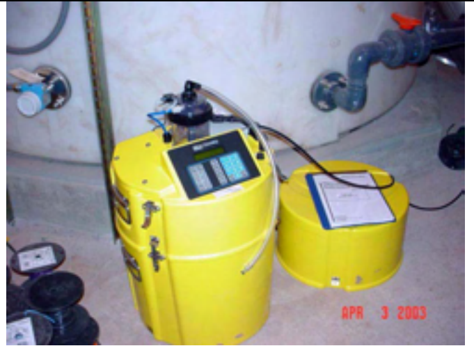
Picture No.: 300 Date Taken: April 3, 2003 Description: Auto sampler for effluent discharge.
