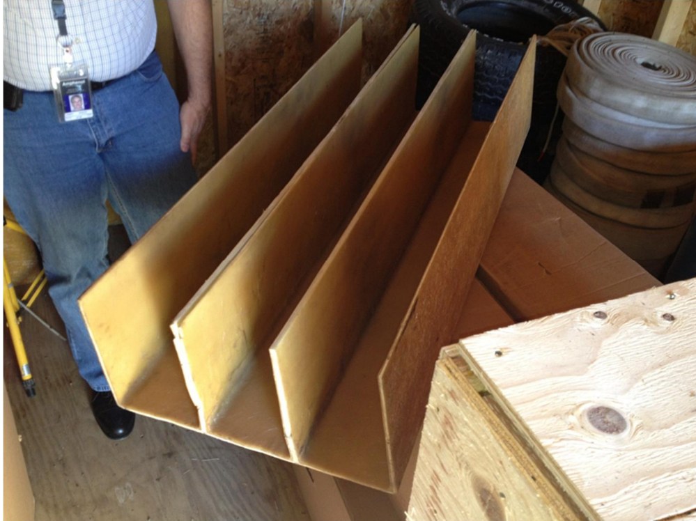
Photo 1 – Typical fiberglass conveyance trench construction
