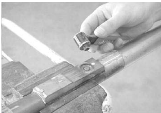
Figure 8.1: Unthread the membrane from the probe block.
