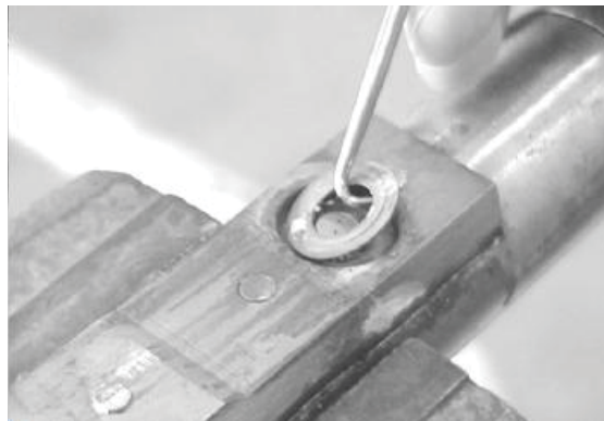
Figure 8.2: Remove and discard the copper washer.
