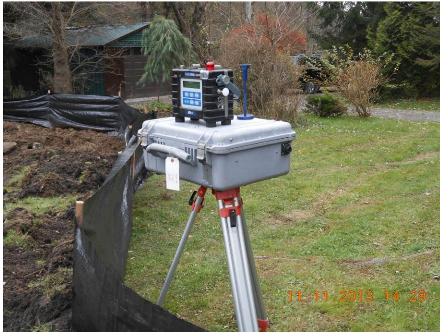
Photo 1: RST 2 deployed three air monitoring stations during Removal Action activities at the Site. Each station comprised of one DustTrack II and one AreaRae air monitoring unit.
