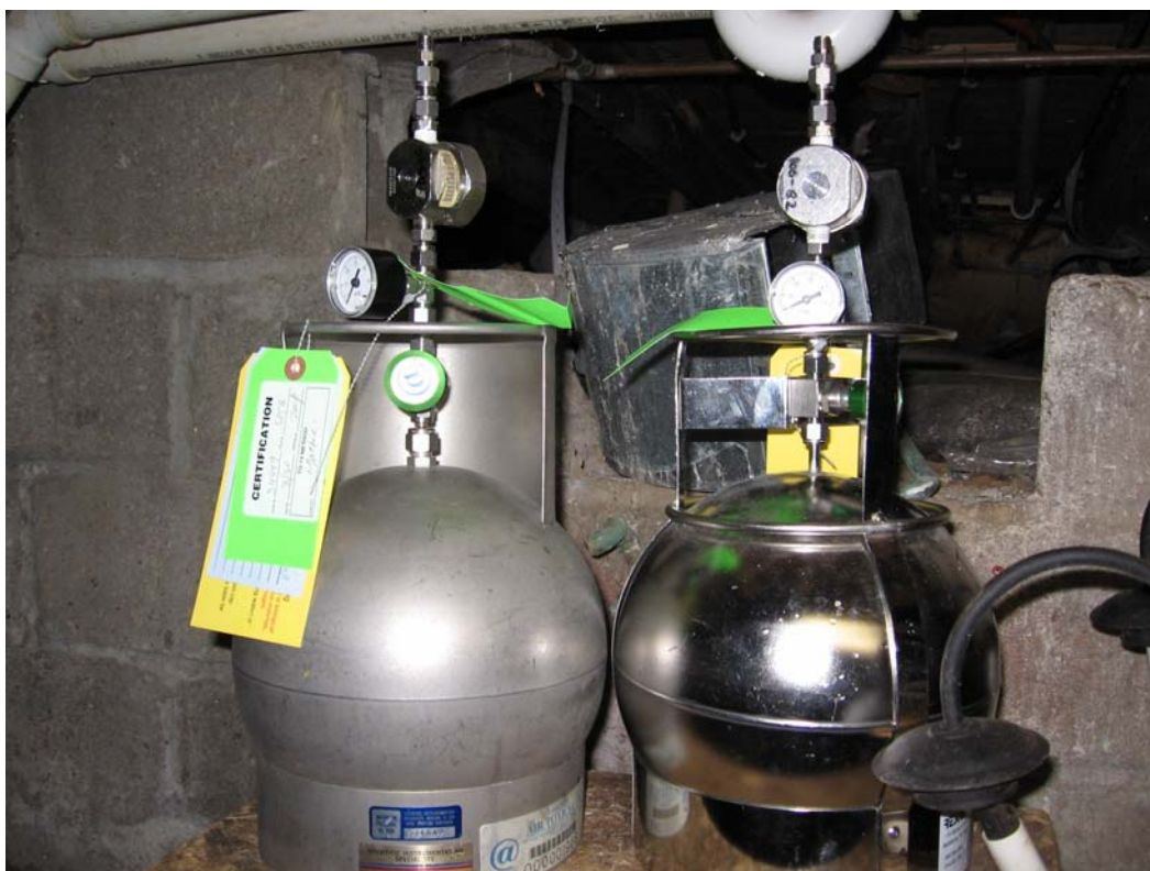
Basement Air Duplicate Sampling Setup at V-2.
