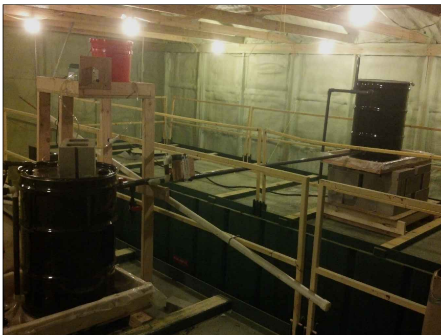
TEST SET-UP (TREATMENT VESSEL ON LEFT, CONSTANT HEAD FEED VESSEL ON RIGHT)
