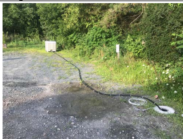
Second injection at INJ-1 by gravity feeding
