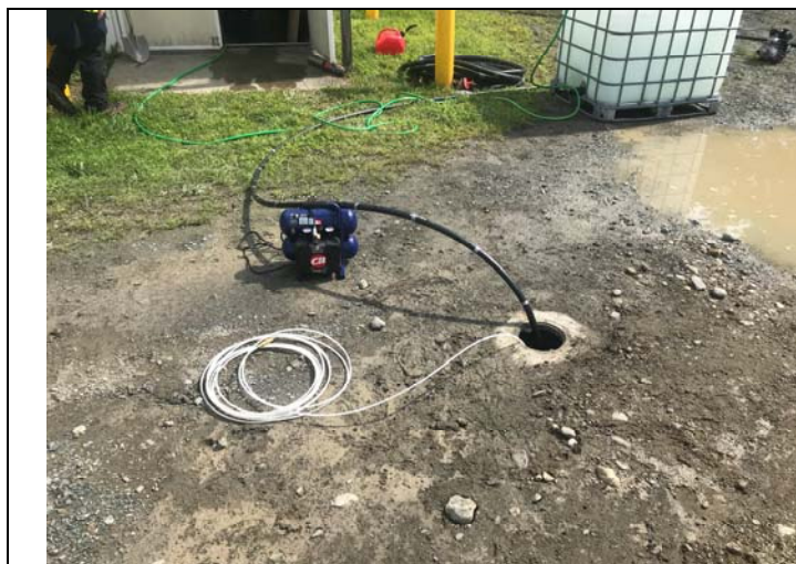
First injection in INJ-2 using packer
