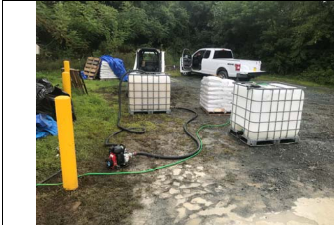
Mixing tank with trash pump and filling other with water from treatment system
