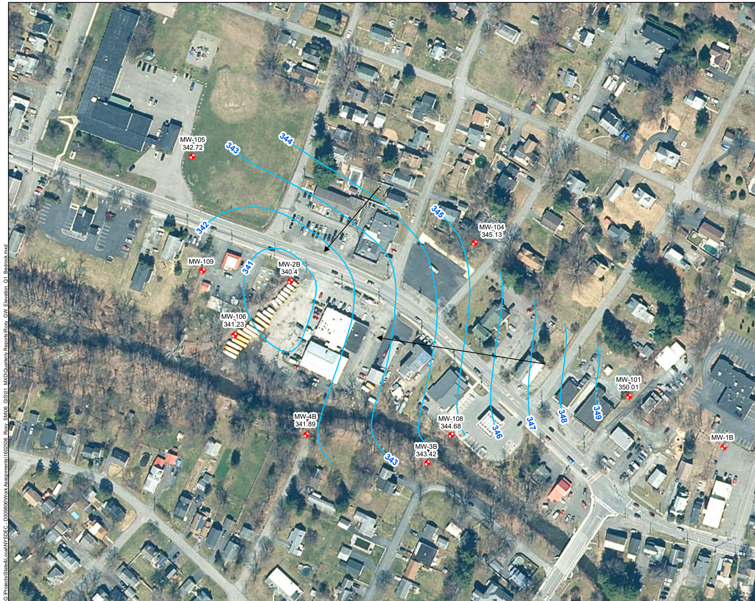
Figure 5 Roxy Cleaners March 2022 Bedrock Groundwater Elevation Roxy Cleaners Site (Site No. 442024) North Greenbush, New York
