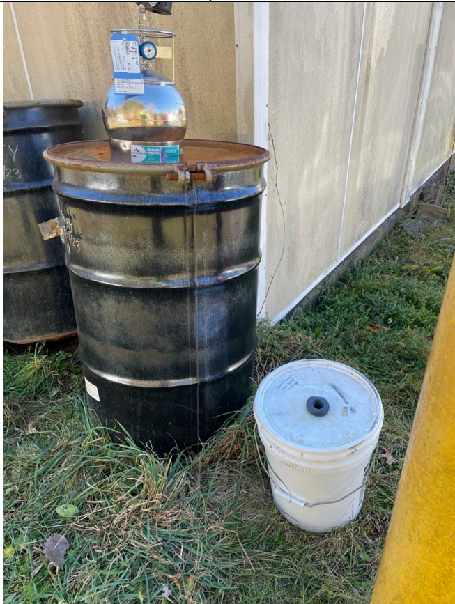
Drum with air can OA-195; carbon bucket used for purge
