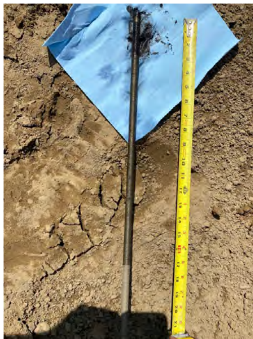
Photograph #60 – Photo depicts contents of 30" bell-spigot pipe – 17 inches of water, 3 inches of dense nonaqueous phase liquid with tar-like odor. (Photo Taken 8/26/2022).
