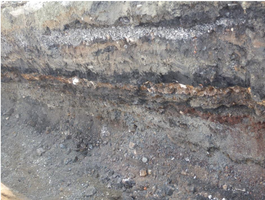
Photo 4. Trench wall with slag levels at bottom. East wall at Station 18+25. View facing northeast.
