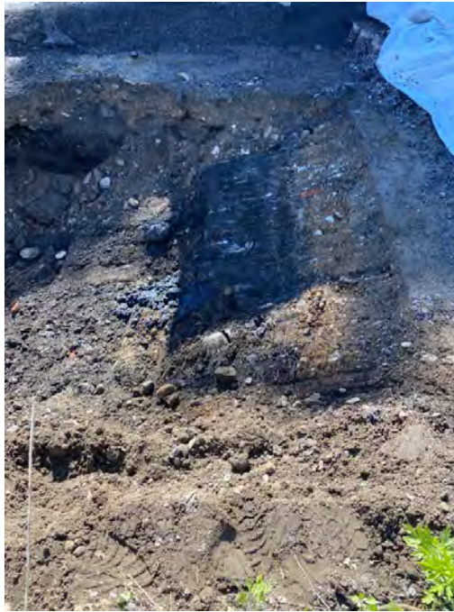
Photograph #39 – View looking west. Photo depicts a layer of tacky tar-like material approximately 1 ft. bgs at test pit completed at Sta. 22+53 on CSX property. (Photo Taken 6/10/2022).
