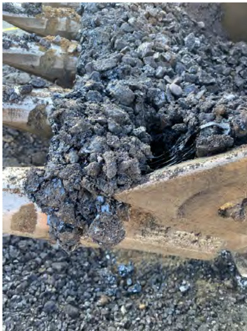
Photograph #46 – Photo depicts tar-like material observed on Area 2 at approximately Sta. 09+80. Tar-like material approximately 18 inches bgs, 6 inches thick, and intermixed with aggregate. (Photo Taken 7/20/2022).
