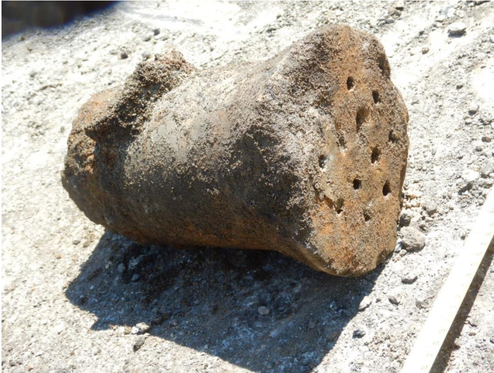
Photo 12. Tuyère variety found south of Station 15+80 and in Area 3. It has 12 holes, measures about 8 inches in diameter at its widest, and is 9 inches long.
