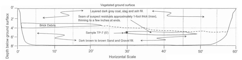
Notes: Suspect residuals consist of dark brown, densely matted wood chips with sulfurous odor. Sample TP-7 (5') collected at 14:00 from depth of 5 ft bgs at distance of 30 feet from the west end of the test pit.
