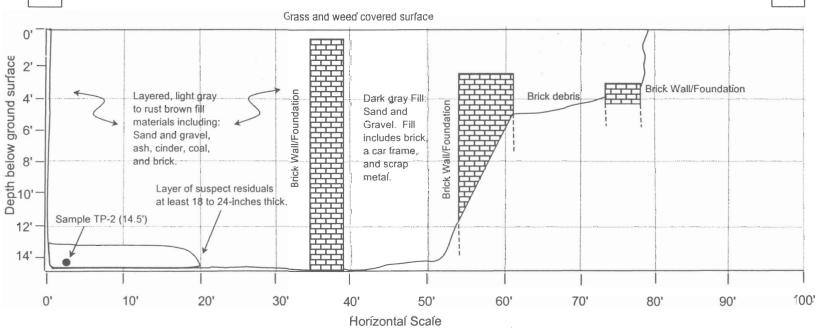
Notes: Suspect residuals consist of dark brown, densely matted wood chips with sulfurous odor. Sample TP-2 (14.5') collected at 11:15 from depth of 14.5 ft bgs at distance of 2.5 feet from the east end of the test pit.
