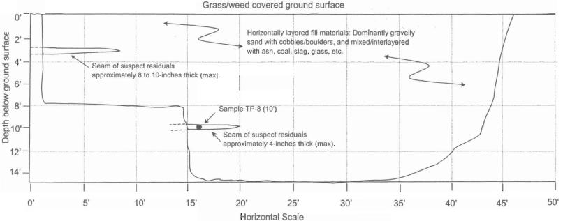
Notes: Suspect residuals consist of dark brown, densely matted wood chips with strong, sulfurous odor. Sample TP-8 (10') collected at 16:00 from depth of 10 ft bgs at distance of 16 feet from the west end of the test pit.
