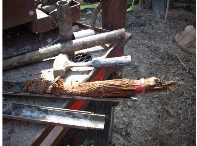
First attempt at IW-A6 Wood in 5 to 7' bgs Split Spoon Found below 1.5 ft of Concrete
