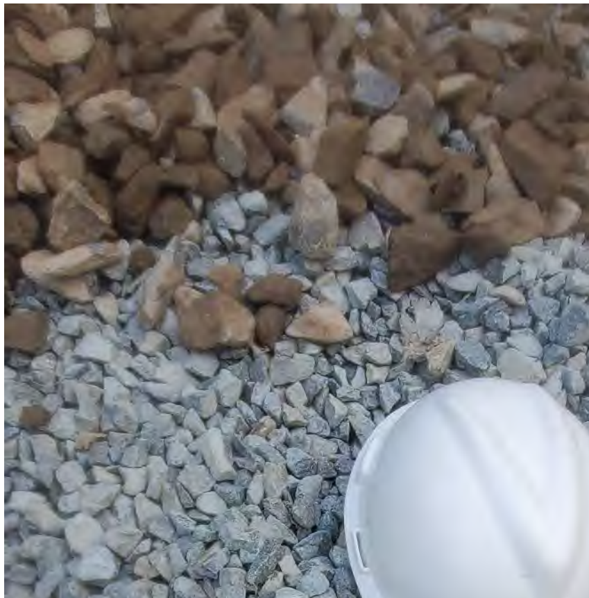
Photo 2: Showing comparison of #2 stone vs #3 stone placed at access road entrance (hard hat provided for scale)
