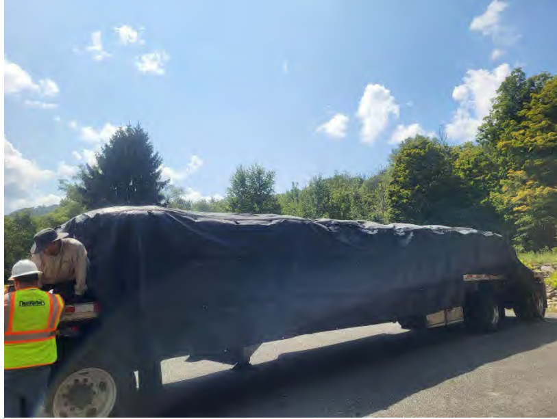
Photo 3: 19 Power Pellet pallets loaded onto flatbed tractor truck and covered with tarp (ratchet straps not pictured)
