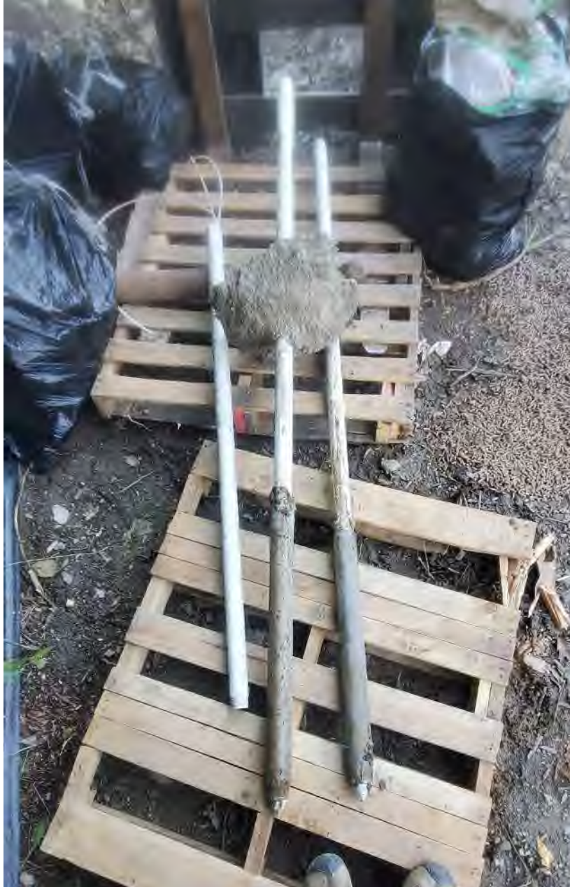
Photo 5: Monitoring wells removed from swale excavations along north side of Building I
