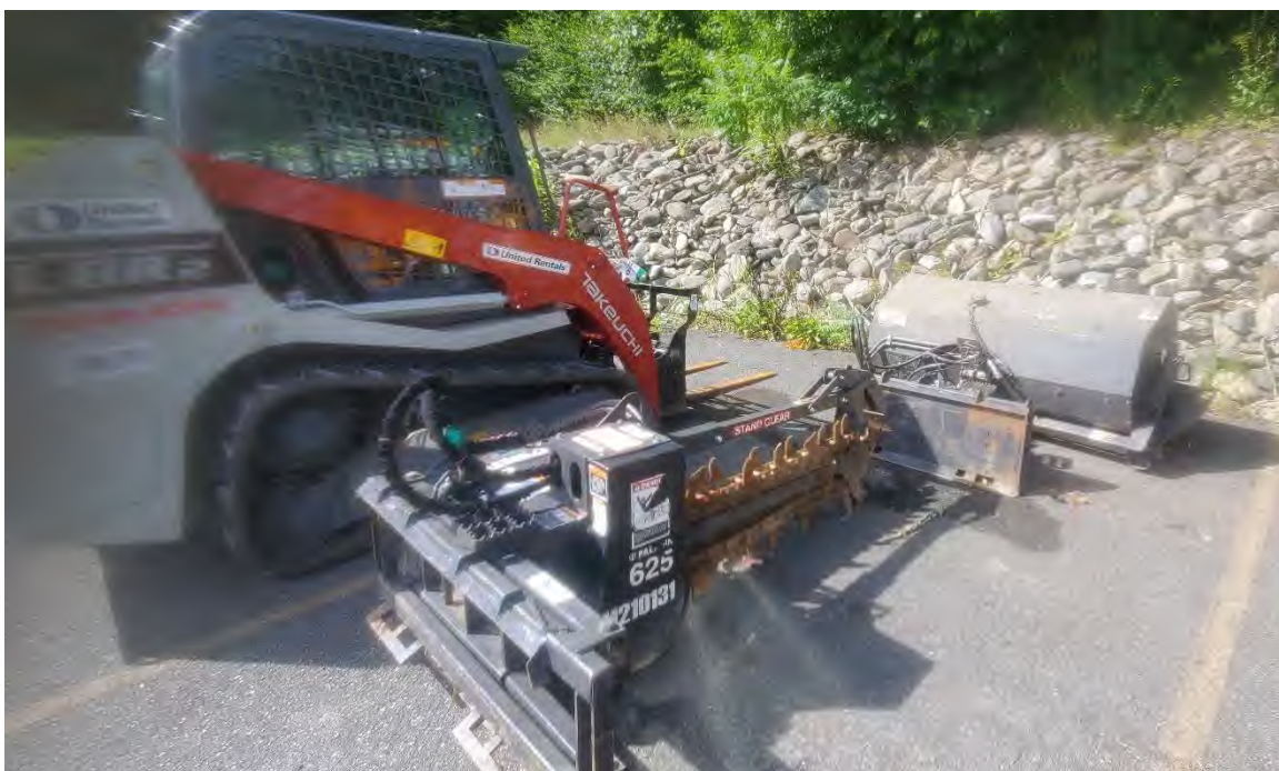
Photo 2: Skidsteer with Forks, Trencher, Brush Roller Attachments
