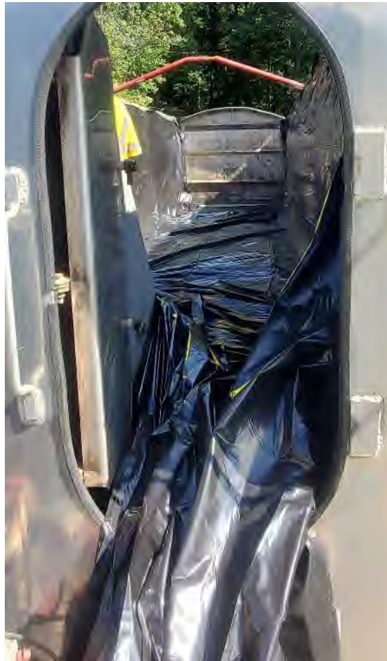
Photo 2: Haul truck lined with poly sheeting prior to loading
