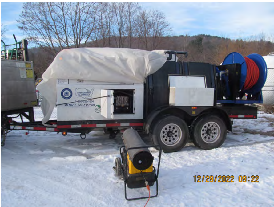
thawing jet unit
