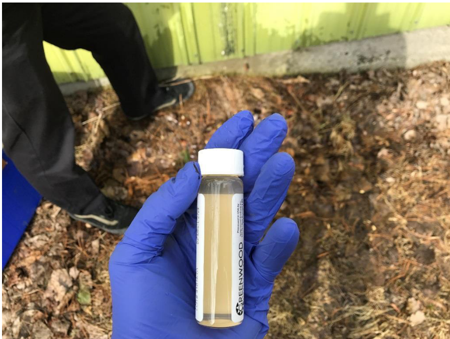
Photograph 2: View of tap water sample collected by RST 3 personnel for target compound list (TCL) volatile organic compound (VOC) analysis. Tap water samples were also collected for TCL semivolatile organic compounds (SVOCs), and polychlorinated biphenyls (PCBs).
