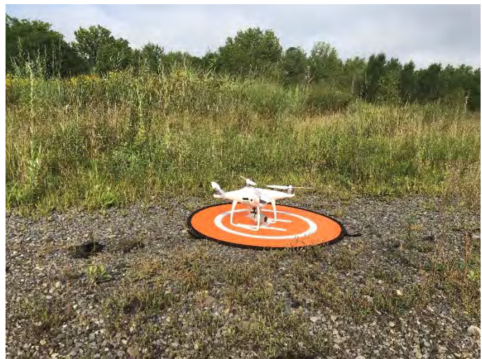
2. Unmanned aerial vehicle (UAV) used to collect aerial photography of the Site.
