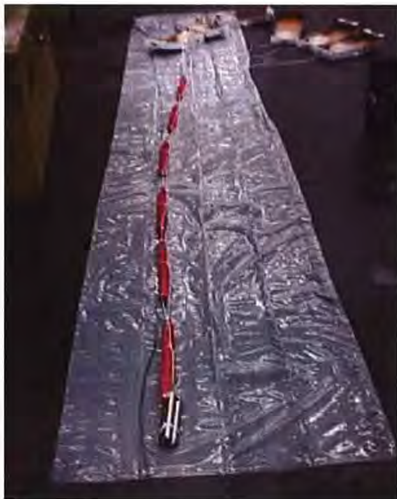
Figure 2. Example of multiple PDB samplers prepared for deployment.
