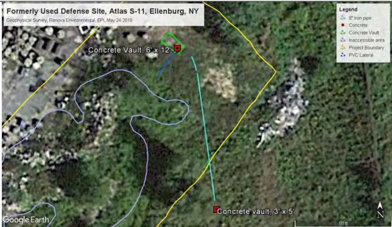
Airborne photo of the northeast end of the survey area shows the two concrete vaults and the pipe connecting them.
