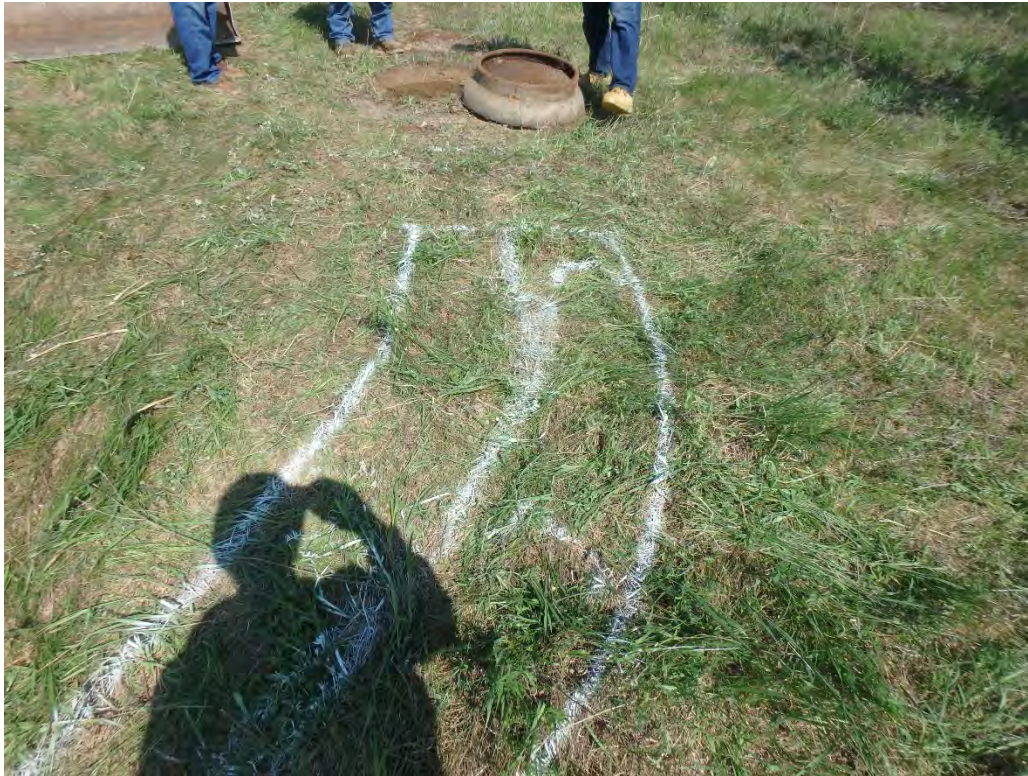
Photo 9 – Piping identified during GPR survey, May 2018
