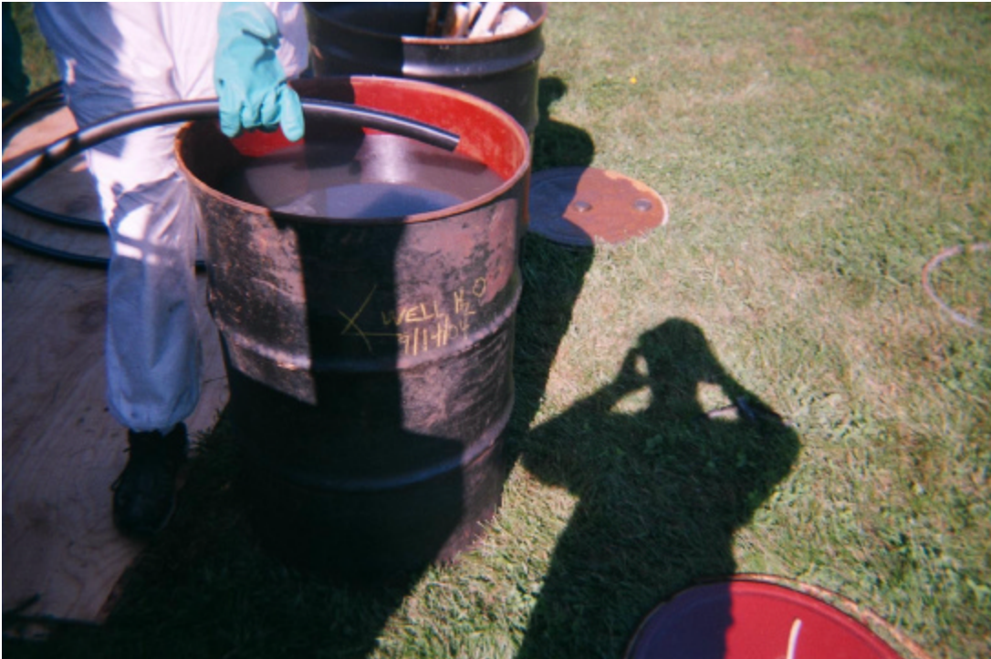
Photo 11: Purge water drum from Angle Well.
