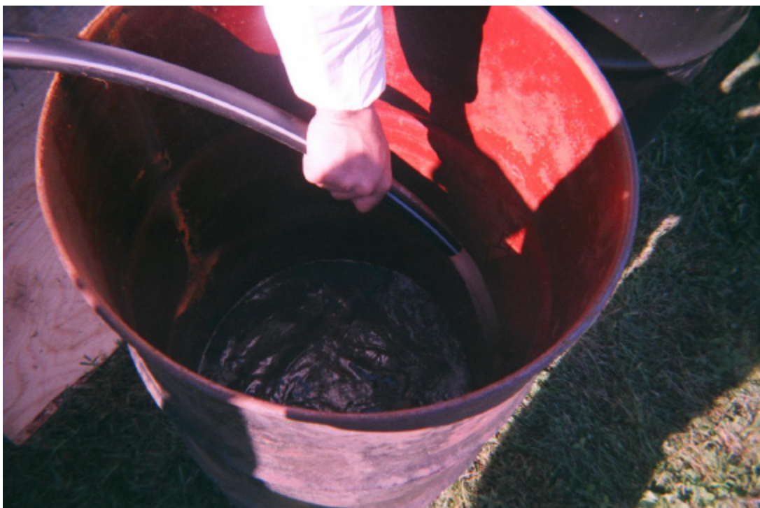
Photo 9: Purge out standing water in Angle Well.
