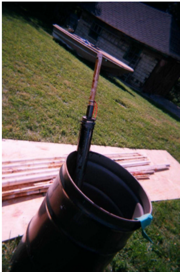
Photo 2: Packer removed from Angle Well.
