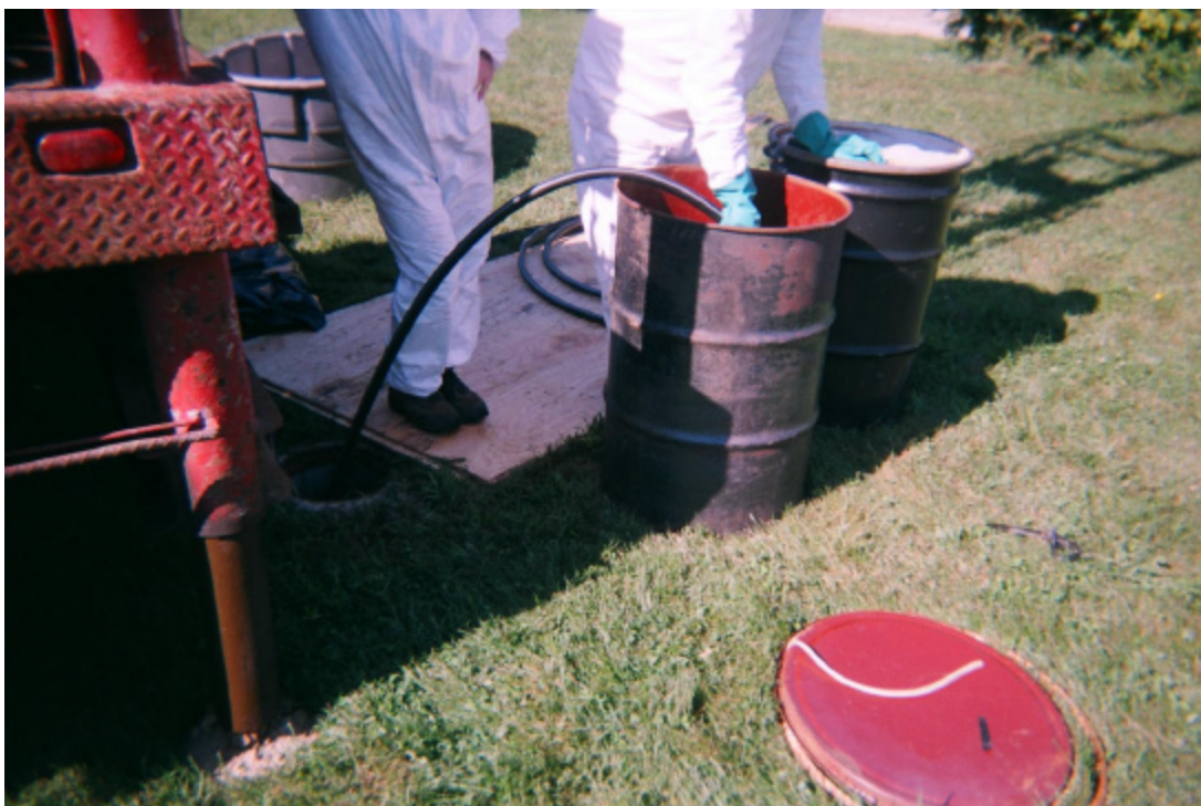
Photo 10: Purge out standing water in Angle Well.
