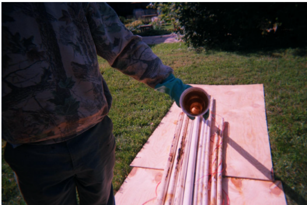
Photo 6: View of inside of 2" PVC (above packer) from Angle Well.
