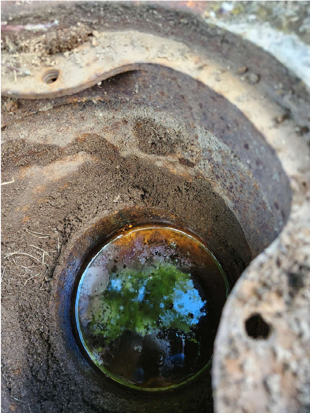
Photo 3: Iron and organic film n MW-9B
