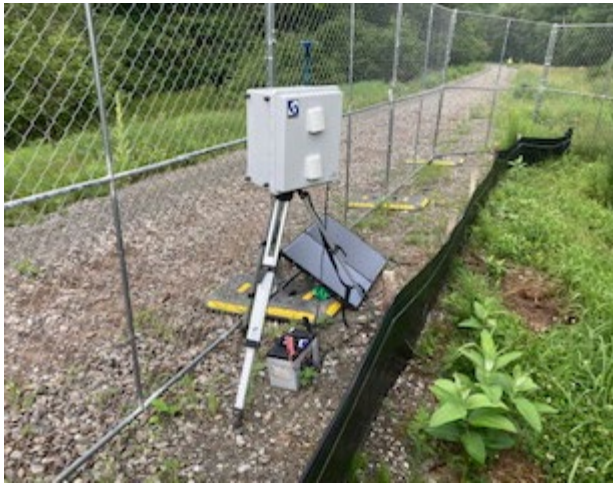
Perimeter air monitoring station along the fence line.
