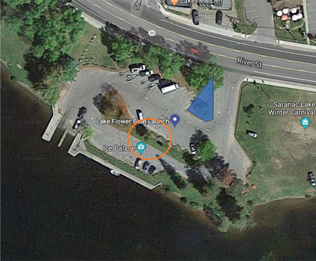
Figure 1. Field Order 13 Item 1: Pave the area shown in blue. Item 2. Grade the area within the orange circle.
