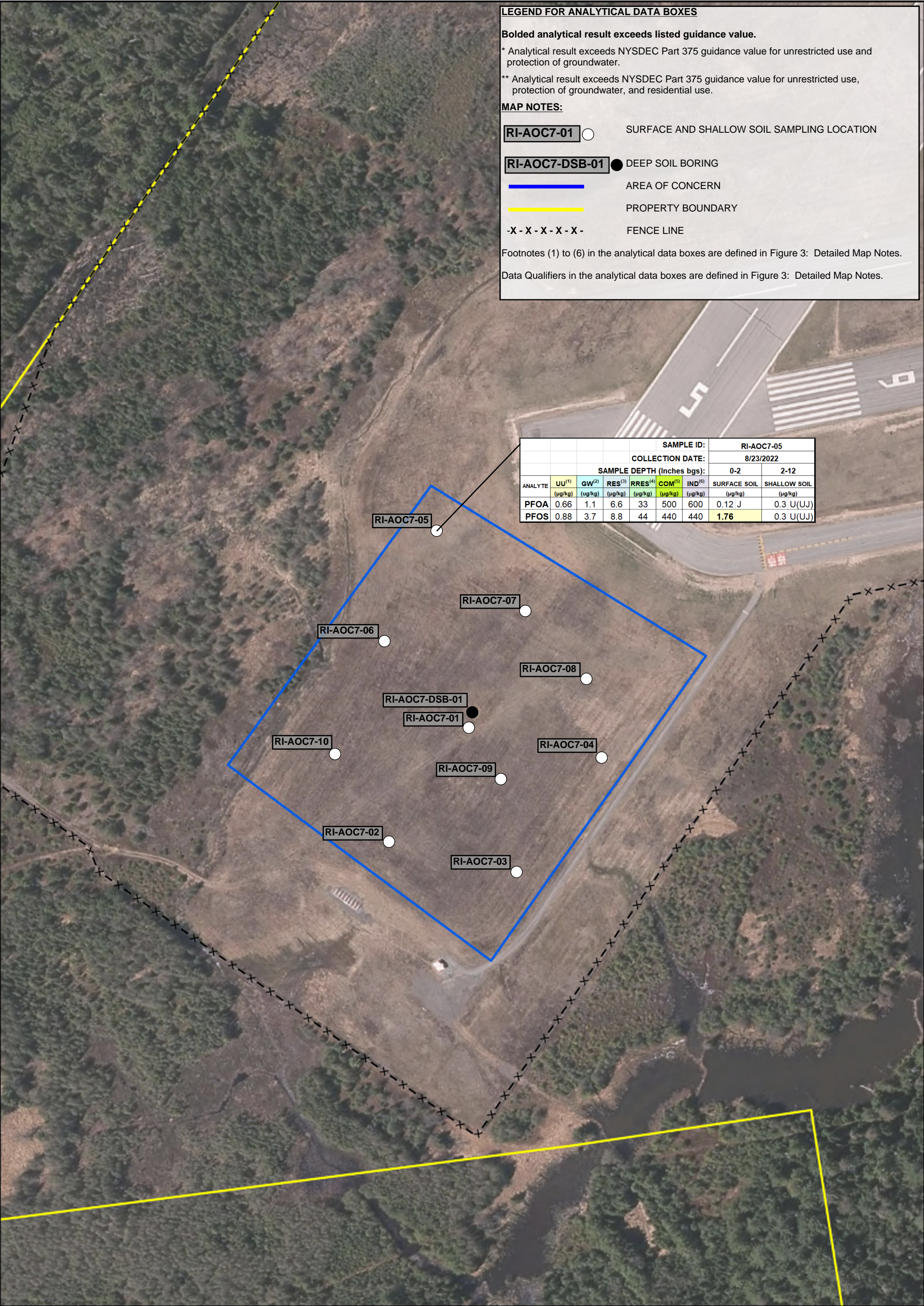
FIG. 13: PFAS ABOVE SCGs IN SURFACE AND SHALLOW SOIL (AOC-7)
